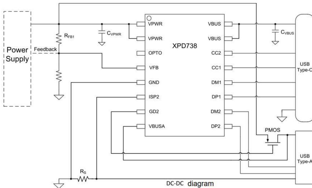
XPD738's built-in Type-C protocol can support automatic wake-up when type-C devices are inserted, intelligently identify the positive and negative of
